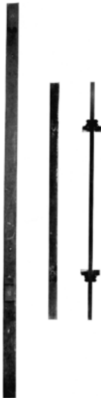
Figure 15.—ONE OF FRANCIS BAILY'S PENDULUMS ( 62\frac{1}{2} inches long), shown on the left, is now in the possession of the Science Museum, London, and, right, two views of a similar pendulum ( 37\frac{5}{8} inches long) made in the late 19th century by Edward Kübel, Washington, D.C., which is no. 316,876 in the collection of the U.S. National Museum. Among a large number of pendulums tried by Baily in London (1827-1840), was one which resembles the reversible pendulum superficially, but which is actually an invariable pendulum having knife edges at both ends. The purpose was apparently economy, since it is equivalent to two separate invariable pendulums. This is the type of pendulum used on the U.S. Exploring Expedition of 1838-1842. It is not known what use was made of the Kübel pendulum.
