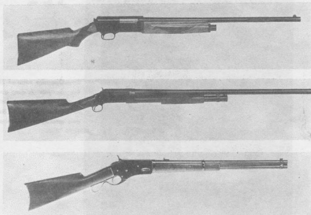
Three guns which incorporated Burgess design or patent features — top, Winchester Model 11 autoloading shotgun; next, Winchester Model 1897 slide action smoothbore and, last, the Whitney-Kennedy carbine (also made in rifle style).
